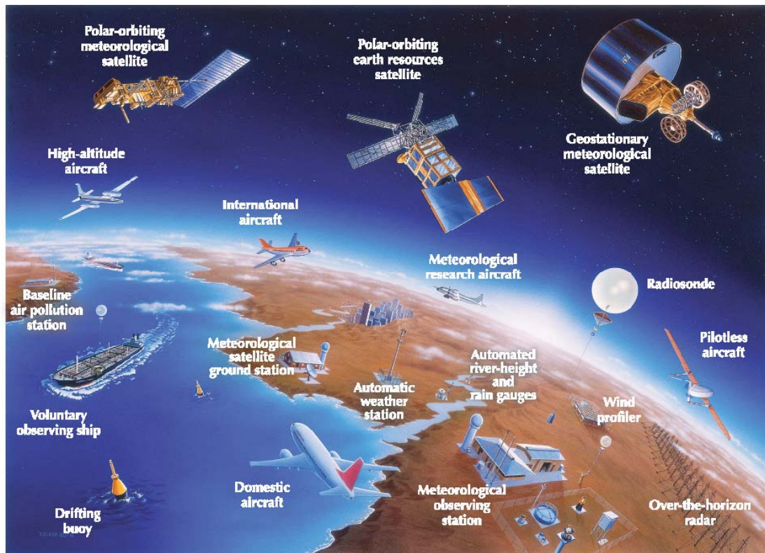
Figure 2.1 Schematic showing a variety of observation systems of relevance to National Meteorological and Hydrological Services. Observation networks rely heavily on the cooperation of many individuals and organizations, many of them volunteers. (Source: Bureau of Meteorology, Australia)
