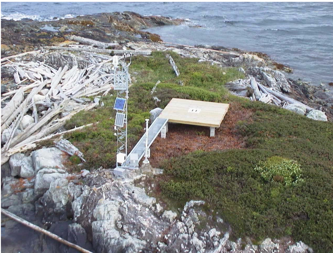
Figure 6.2. A remote coastal automatic station showing helicopter landing pad and other features such as solar panels. (Source: Meteorological Service of Canada)
