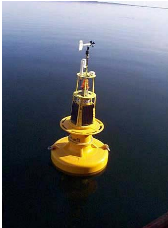
Figure 6.5. A moored 1.7 metre buoy employed in part of the Canadian network. (Source: Meteorological Service of Canada)
