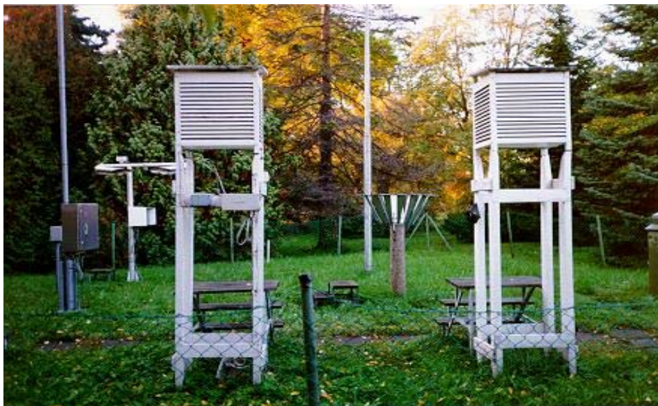
Figure 6.7. Old and new side by side. Comparison data being collected at Helsinki to ensure continuity and homogeneity of climate records collected from the former manual station, which operated from 1844. (Source: Finnish Meteorological Institute, Finland)
