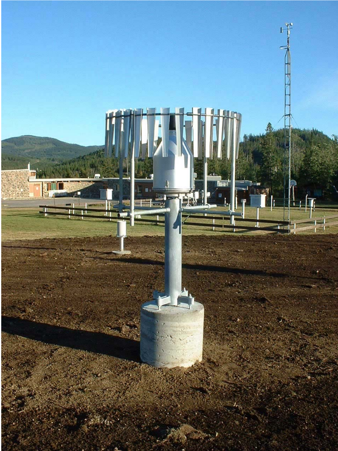
Figure 6.4. An all weather precipitation weighing gauge. This particular one is a Geonor T-200, used by a number of meteorological services. (Source: Meteorological Service of Canada).
