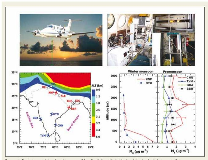
Top panels: The instrumented aircraft used to measure BC profiles (left) and the inside view of the aircraft with instruments. Bottom Panels: Locations of aircraft measurements of BC with aircraft symbol (left). The altitude distribution of BC over Indian region during winter and pre-monsoon seasons (right panels).
