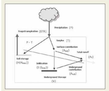
The Temez conceptual model: A surplus (T) part of the water which precipitates (P), is infiltrated (I) to the second layer, and goes to the stream-flow (Asup), whiles the rest of this water (P) is stored in the first layer of soil. Here, evapotranspiration occurs and the soil may also store water from one month to another. In the second layer, the water can drain to the stream-flow and may also be stored
