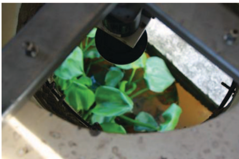
Photo TI3.7.1 Vegetation obstructing water-level measurements.
