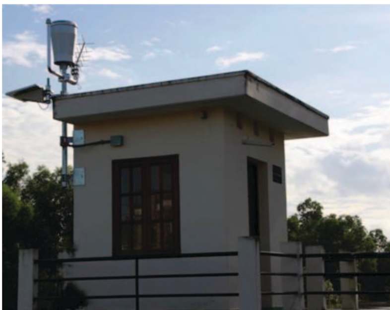
Photo 3.2 River gauging housing located on a tributary of the Mekong River, near Ho Chi Minh City, Vietnam. A rain gauge, satellite communication antenna, and solar panels are located on the roof.
