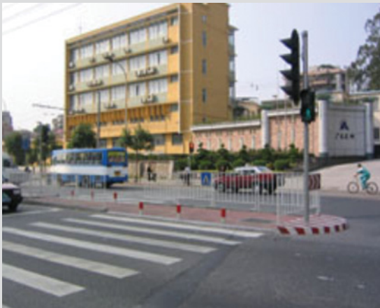
Figure B10.6.2 Staggered Pedestrian Crossing
