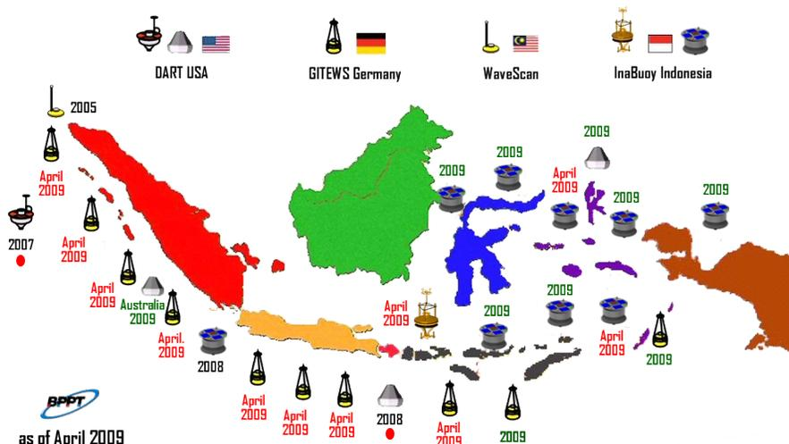
Figure 6.4 IOTWS and Ina-TEWS Tsunameter Array
