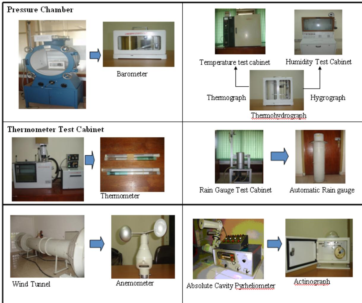
Figure 7.1 Facilities for calibrating meteorological observation instruments
