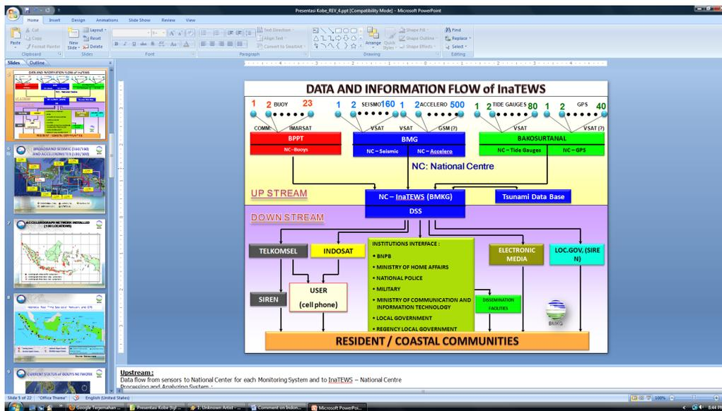
Figure 5.2 End-to End Tsunami early warning system
