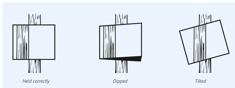
Figure 5.14 Observing a tree stem through a stick-type angle gauge
