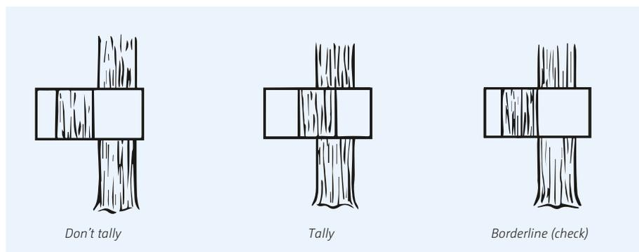
Figure 5.13 Holding the wedge prism correctly
