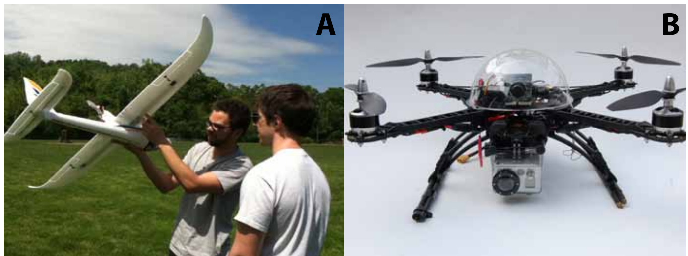
Figure 5.1. Types of unmanned aircrafts (drones). A. Fixed wing; B. Multicopter.
