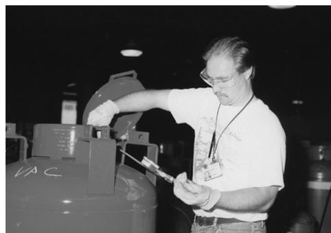
Photo 7-2. Conducting a temperature-pressure test.
