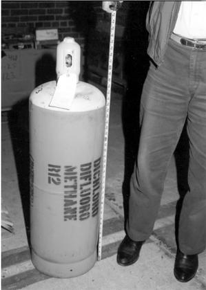
Photo 6-9 - Example of CFC-12 cylinder, dichlorodifluoromethane.
