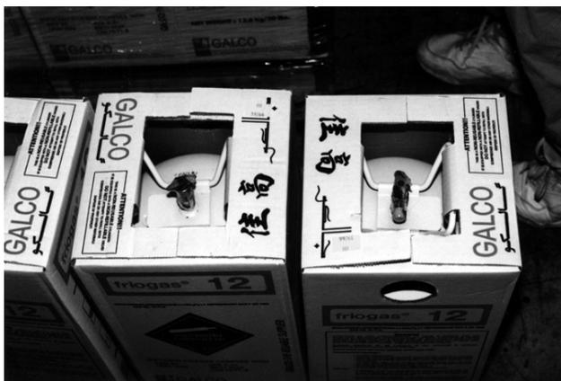
Photo 6-5 - Cardboard packaging for 13.6kg (30 lb) disposable cylinder, top view.
