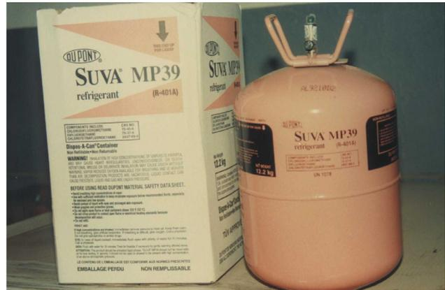
Photo 6-2 - Disposable cylinder with SUVA MP39 - an R-401 refrigerant blend containing HCFCs.
