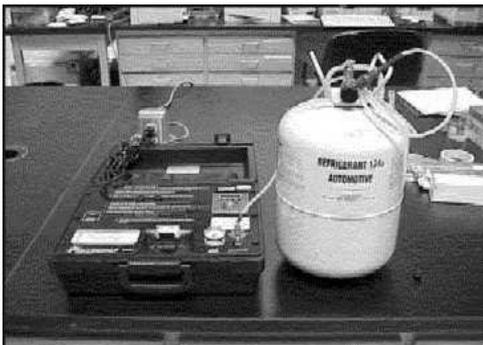
Refrigerant identifiers/analysers are small portable units used to identify certain ODS and non-ODS. The more sophisticated models detect CFCs, HCFCs, HFCs and hydrocarbons. They are also able to analyse the composition of certain refrigerant blends, their water content, and purity and to indicate the presence of highly flammable substances.
