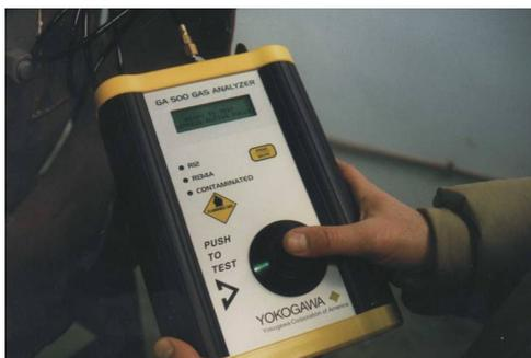
Portable identifiers/analysers are connected to the cylinder or equipment; they do not require samples. Therefore, any trained Customs personnel familiar with the use of refrigerant identifiers/analysers can test the refrigerant charge of cylinders and certain stationary and mobile air-conditioning systems.
