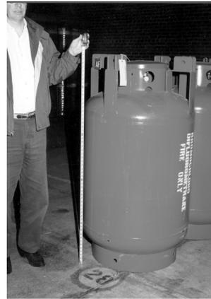
Photo 6-22 - Cylinder of halon 1211 (bromochloro difluoromethane).
