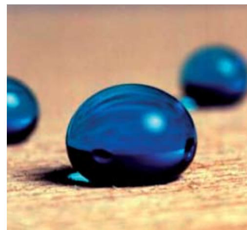
Wood coated with a nanoparticle surface becomes extremely water repellent or 'superhydrophobic'. Surfaces treated in this way become self-cleaning and require little maintenance.
