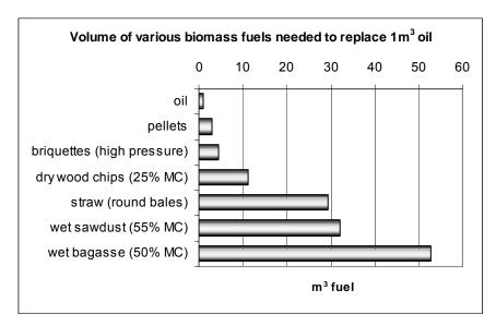
Figure 4: Volume of biomass fuels equivalent to 1 cubic metre of oil7
