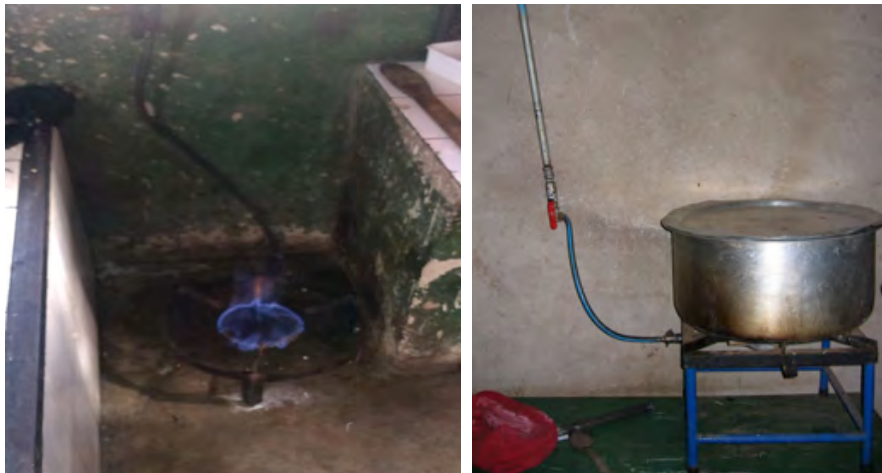
Figure 10: Gas cookstoves designs are currently not sufficient for large volume saucepans
