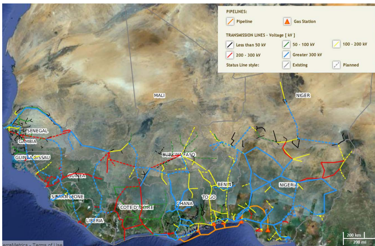
FIG. 23. Transmission lines and gas pipeline in West Africa. (Reproduced courtesy of ECREEE ECOWREX [42])
