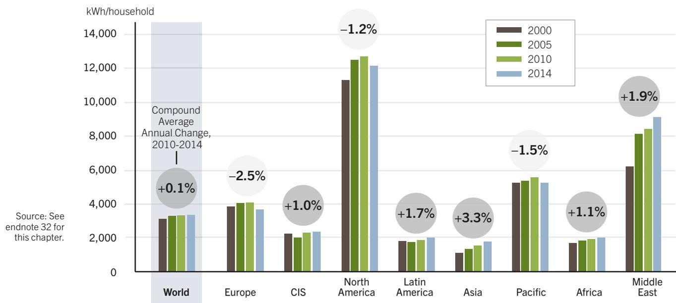
Electricity accounts for nearly one-third of global TFEC in the buildings sector. Electricity consumption per household is used as an indicator to suggest trends in the efficiency of electricity use at the global and regional levels; however, this does not isolate the effect of improved efficiency from the effect of changes in demand for electricity services.
