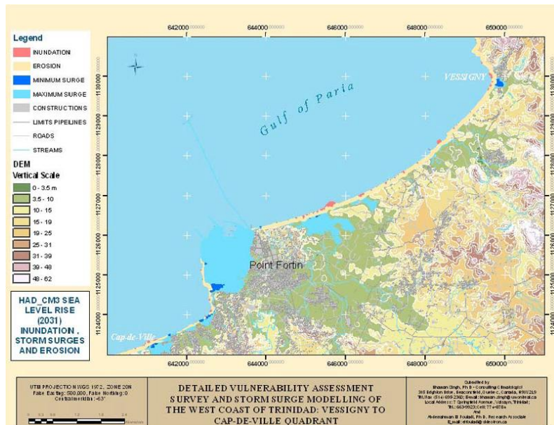
Inundation And Erosion Of The Coastland Along The Gulf Of Paria On The West Coast Of Trinidad Due To Sea Level Rise As Simulated By Hadcm3 And Flooding Due To Minimum And Maximum Storm Surges, Coupled With The Dem, 2031 :Vessigny To Cap-De-Ville Quadrant (Singh. B. and A. El Fouladi, 2007)
