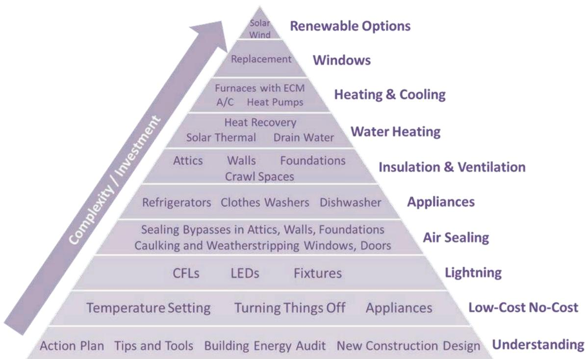
**Figure 7 – Energy-Saving Pyramid – Technical measures**
