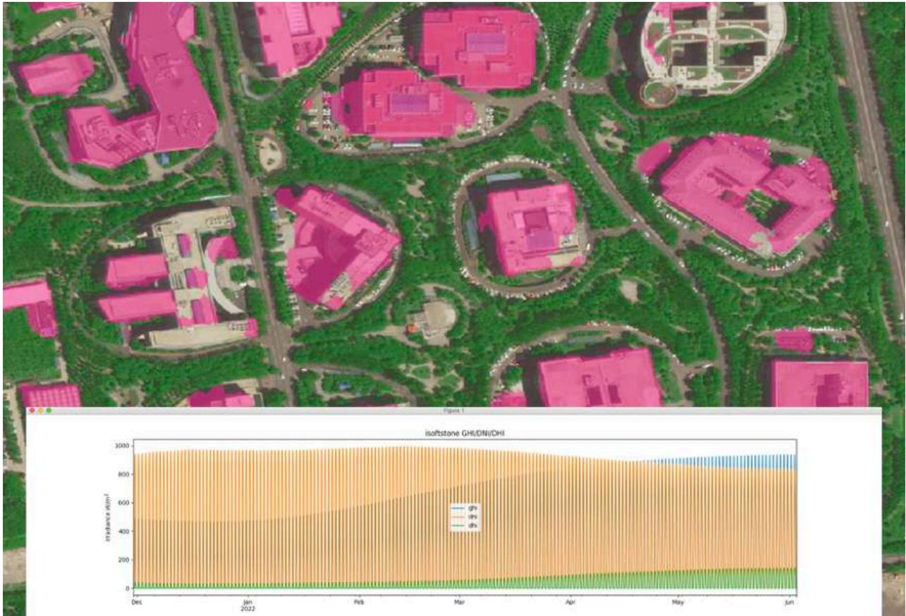
Figure 3-20: AI Roof Area and PV Revenue Measurement System Source: ISSTECH
