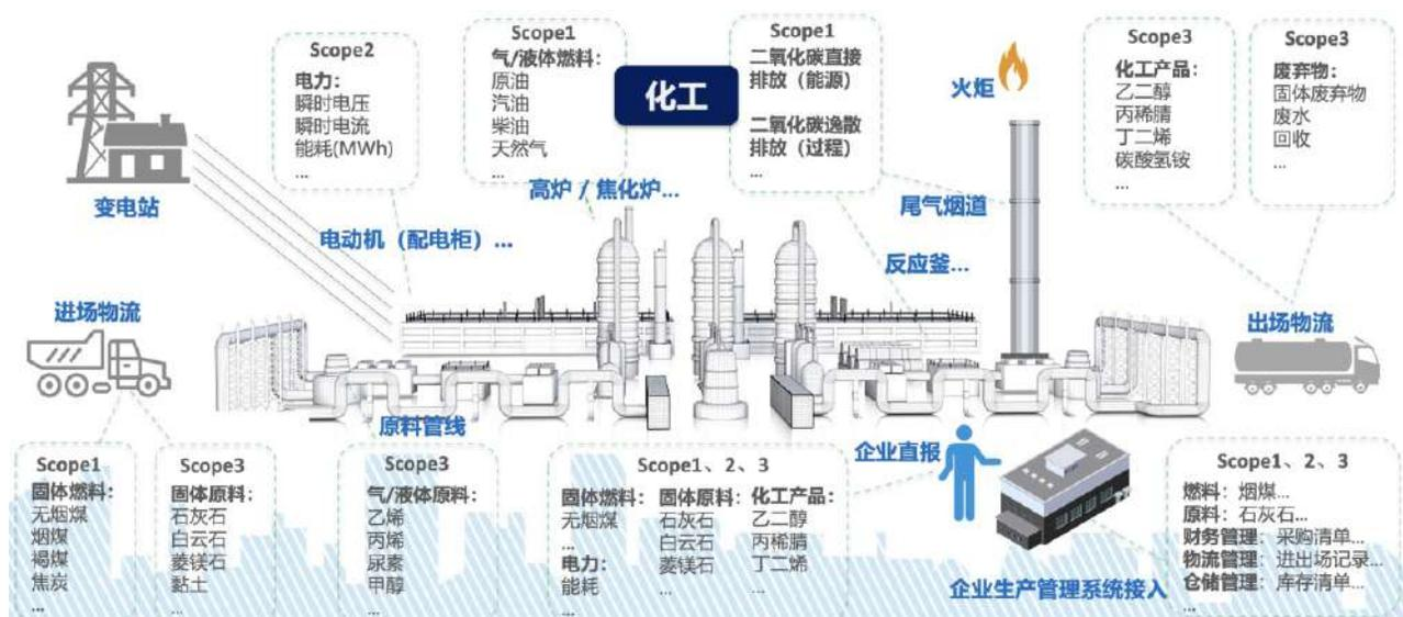
Figure 3-4: diagram of carbon emission monitoring in the chemical (heavy industry) sector Source: draw by author
