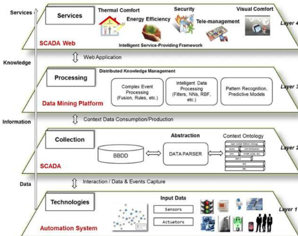
Figure 2-1 common architecture of smart building management system (Moreno et al. 2014)
