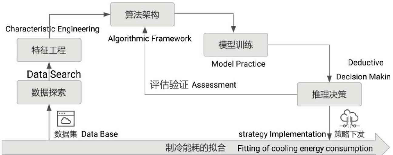
Figure 3-9: High efficiency refrigeration control strategy Source: Next Generation Data Center White Paper, Huawei
