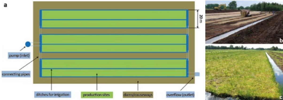
*Sphagnum* farming: a: site with infrastructure for water management (pump, ditches, overflow) and dams used as causeways (maintenance, harvest, transport) (schematic representation: Sabine Wichmann) b: Preparation of a *Sphagnum* farming production site (photo: Sabine Wichmann); c: same site with established *Sphagnum* culture and irrigation system (photo: Sabine Wichmann).
