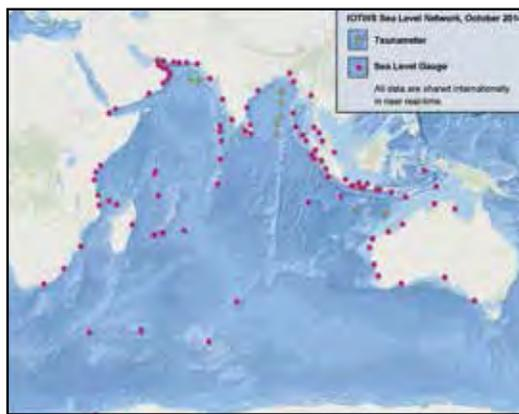
These maps illustrate the improvements between 2004 to 2014 in the core seismic network and the core coastal sea-level station and deep ocean tsunameter networks. Developed as part of the IOTWS, these networks share data regionally and globally in near real time.
