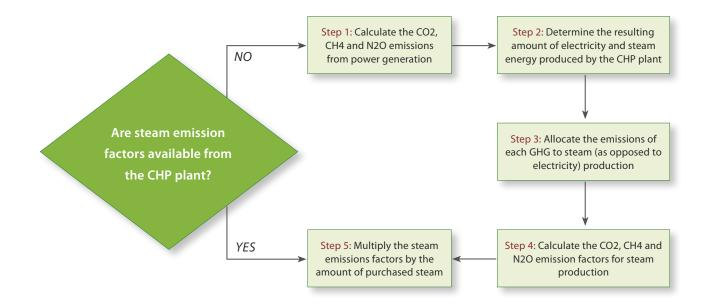
If the energy provider is able to supply emission factors for steam production, proceed to step 5. Otherwise, calculate the emission factors following steps one - four below. Each step should be repeated for each of CO2, CH4 and N2O.
