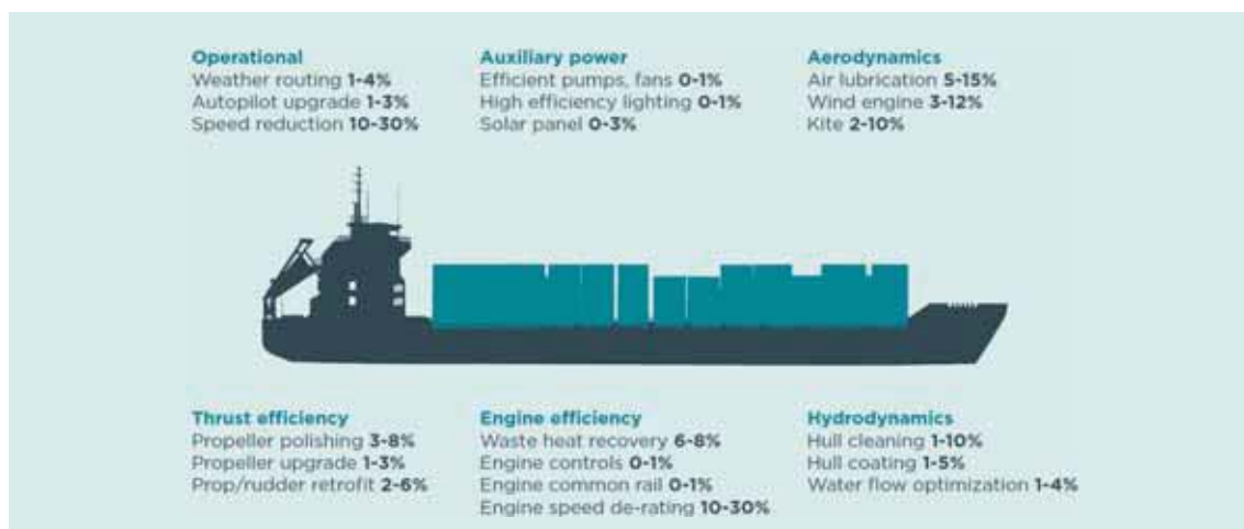
Figure 1. Potential fuel use and CO 2 reductions from various efficiency approaches for ships (International Council on Clean Transportation (ICCT), July 2013). Long-term potential for increased shipping efficiency through the adoption of industry-leading practices. http://bit.ly/17NasAT
