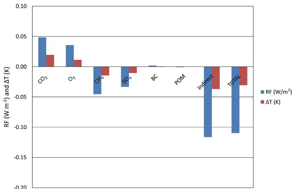
**Figure 8.4** Global mean radiative forcings ( $W m^{-2}$ ) and temperature responses (K) in 2007 from shipping emissions. The figure does not include the positive RF that could possibly occur from the interaction of BC with snow, which has so far not been investigated for ships.
