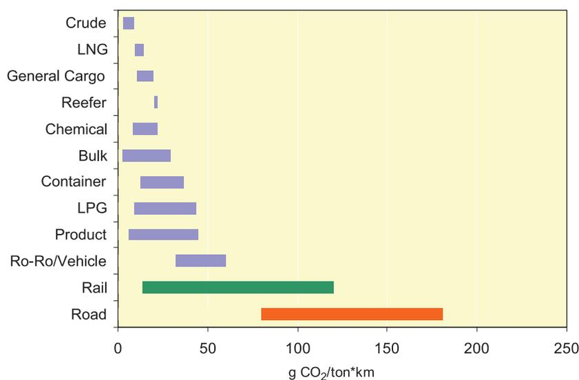
**Figure 9.2** Typical range of ship CO<sub>2</sub> efficiencies compared to rail and road
