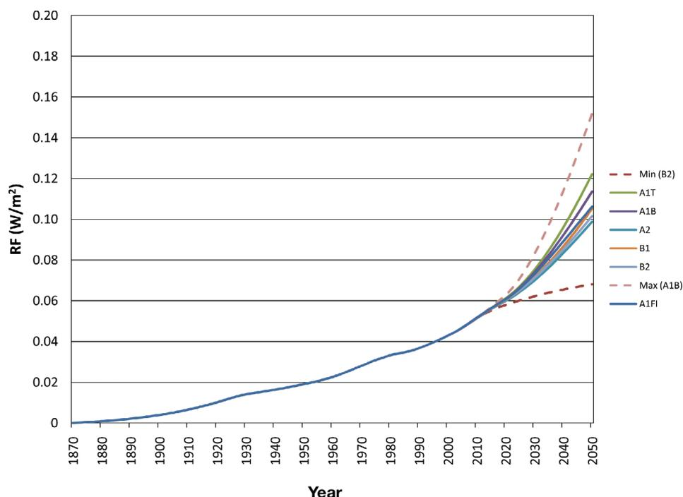
**Figure 8.3** Radiative forcing of CO<sub>2</sub> attributable to shipping from 1870 to 2005, and thereafter, according to a range of scenarios, to 2050
