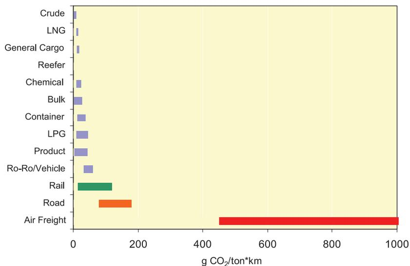
**Figure 9.3** Typical range of ship CO<sub>2</sub> efficiencies compared to rail, road and air freight
