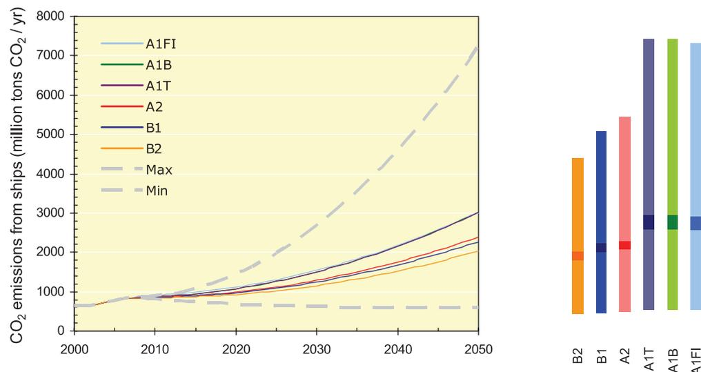
**Figure 1.2** Trajectories of the emissions from international shipping. Columns on the right-hand side indicate the range of results for the scenarios within individual families of scenario.
