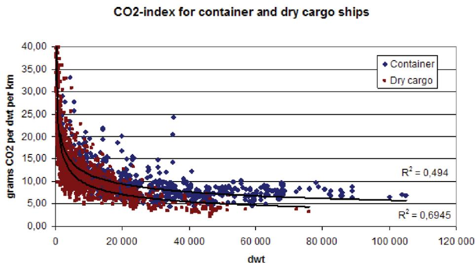
**Figure 6.1** *The effect of ship deadweight on CO<sub>2</sub> design index [2]*
