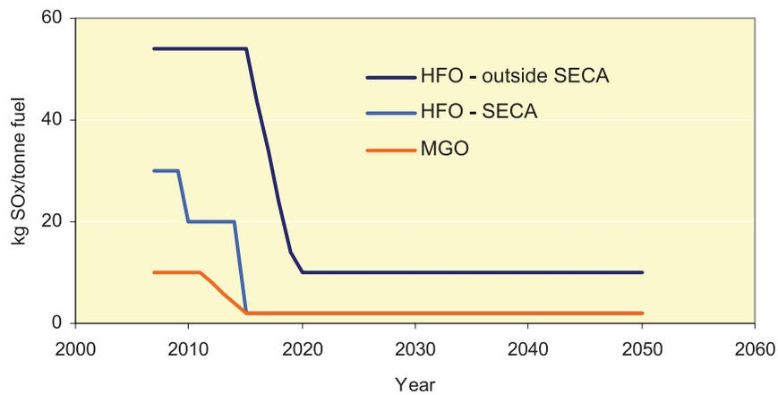
**Figure 7.6** Future  $SO_x$  emission factors used in scenarios. The future limit of 3.50% in 2012 on global sulphur content is not expected to influence the average emission factor
