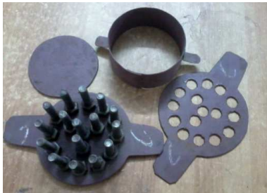
Figure 5. Components of mould for producing beehive briquettes
