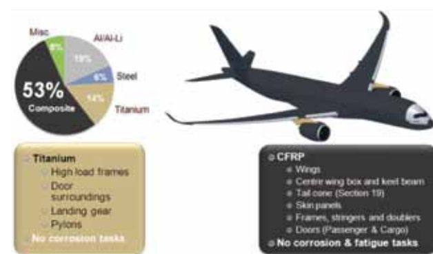
Figure 2: Airbus A350 XWB Airframe Use of Composites.
