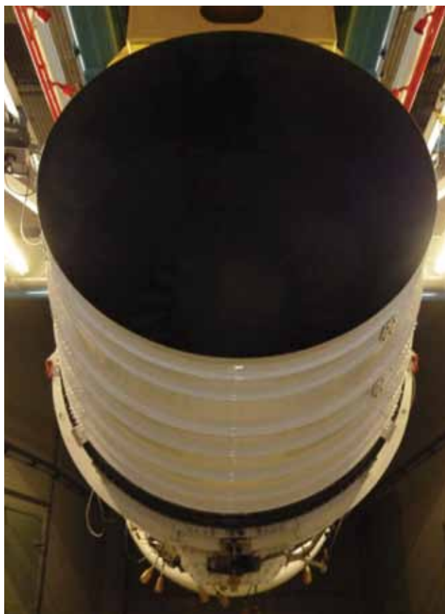
Figure 5: A Validation Issue: Representative Sampling of the Entire Exhaust Plane with Certification Probe Systems.
