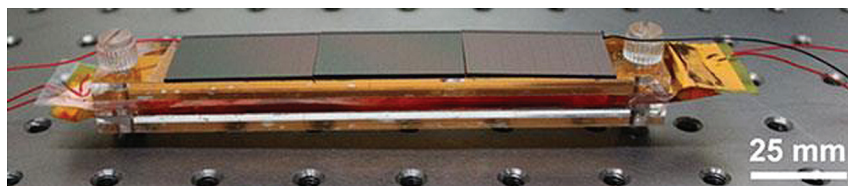
Triboelectric generator that can harvest wind energy.
