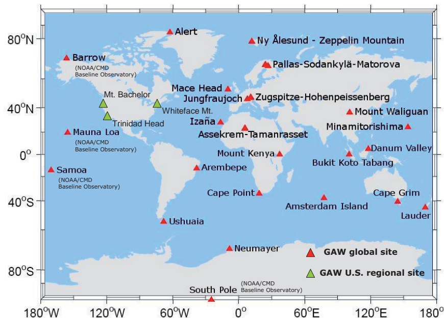
Figure 2.26. Network of surface-based remote observatories organized through the World Meteorological Organization's Global Atmospheric Watch (GAW) Program.
