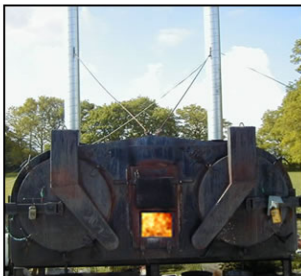
Figure 8. Retort kiln for biochar production
